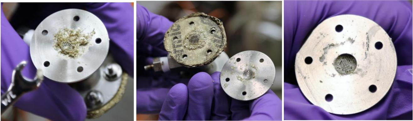
**Figure 10: Aft Diffuser Plate Post Firing Showing Wet Gasket (Left), Front Diffuser Plate Post Firing (Middle), Catalyst Screens with Gasket Residue (Right)**
