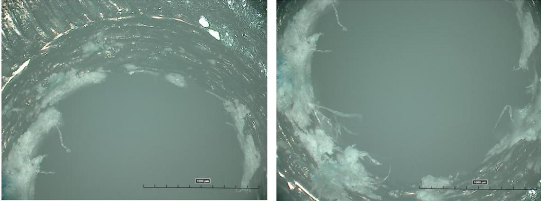
**Figure 11: Non-concentric Throat Top (left), Bottom (right) Radius Before Pulse Tests**
