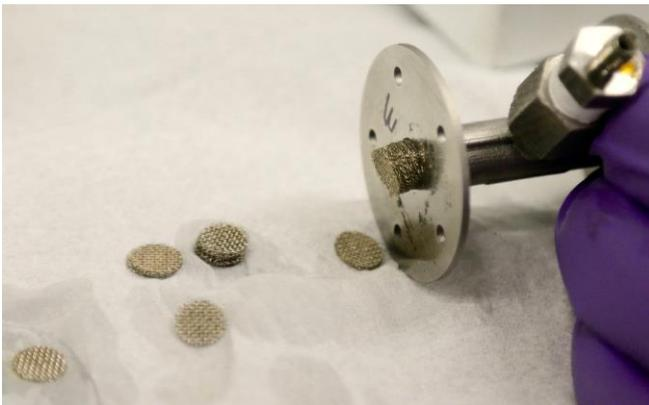
**Figure 9: Disassembling the Catpack Screens**
