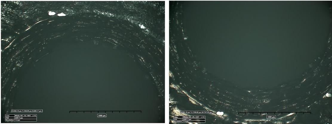
**Figure 12: Non-concentric Throat Top (left), Bottom (right) Radius After Pulse Tests**
