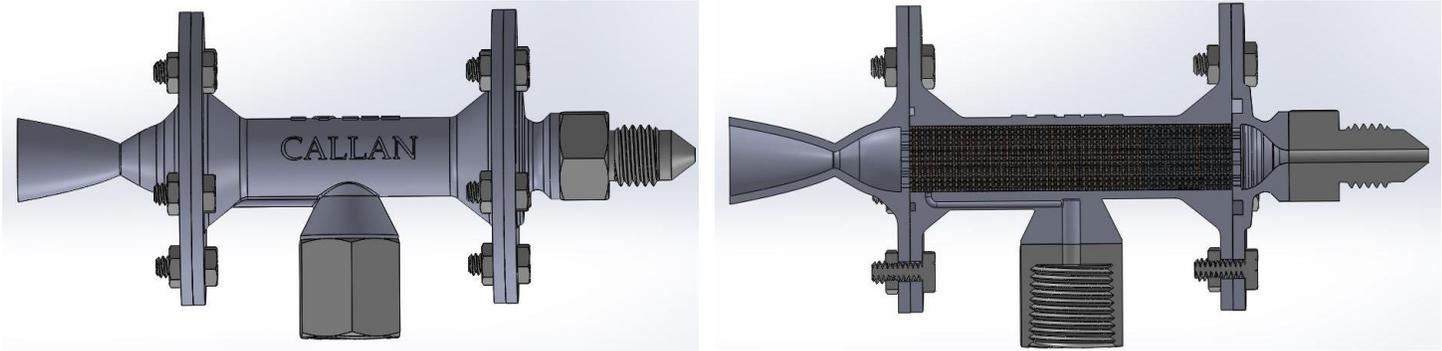
**Figure 1:** A computer generated model of the monopropellant engine, Callan: (a) Exterior view, (b) Interior cross-sectional view.
