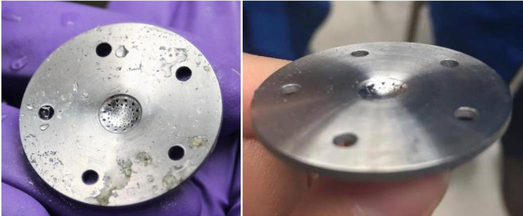
**Figure 8: Deflected Orifice Region After ~1000 lb of Compressive Force**
